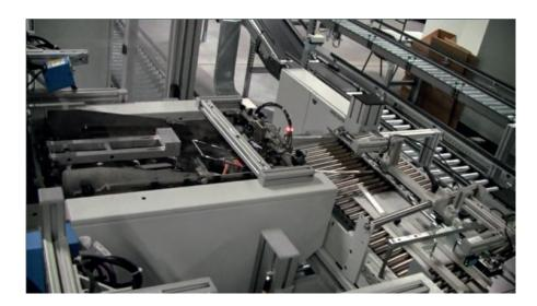
The document feeder ensures uniform document tracking, different packages can be loaded automatically.
